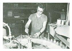
(photo left) BOB BAKER (I), Foreman, shared a production problem with Industrial Engineers OAKLEY CAMPBELL (center) and JOHN STULL (r) who came up with a unique design for an automatic unloader for a rotary buff (polishing) machine used in the manufacturing of Balcrank's solid and revolving handles. (photo right) Due to the elimination of manually unloading the handles, Buff and Polish Operator LARRY DAVIS finds that productivity has increased 300 percent!
